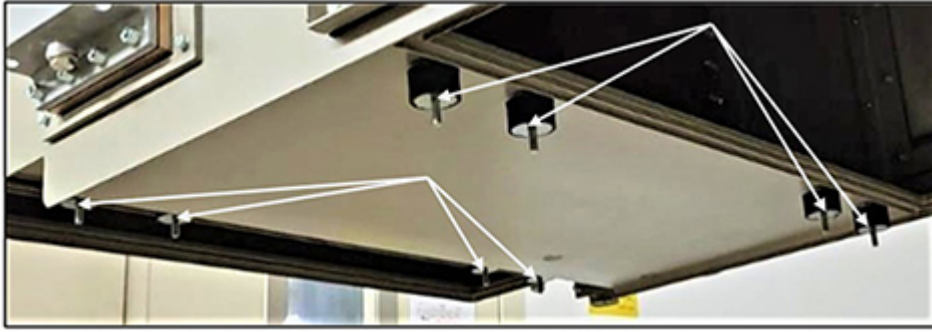
FIGURE 9. 8 X ANTI-VIBRATION MOUNTS INCLUDING 6MM WASHERS FITTED TO UNDERSIDE OF WATER COOLER.
