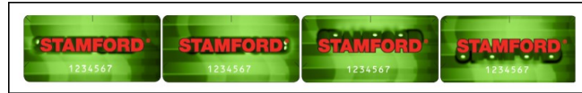
FIGURE 14. DOTS VISIBLE IN LEFT, RIGHT, UPPER AND LOWER VIEWS OF 3D HOLOGRAM
