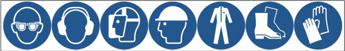
FIGURE 1. MINIMUM RECOMMENDED PERSONAL PROTECTIVE EQUIPMENT (PPE)
